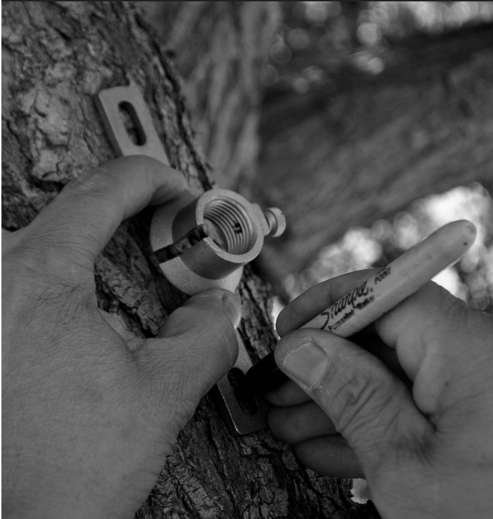
1. Use A Sharpie to mark desired location of the FA-TB2A bracket
