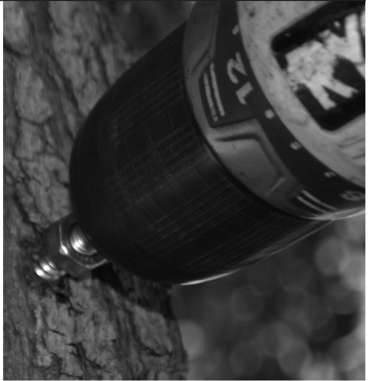
2. Using a Screw Gun attach hanger bolts to the tree Note: You may also use a 7/16" socket wrench and a drill to attach the hanger bolts
