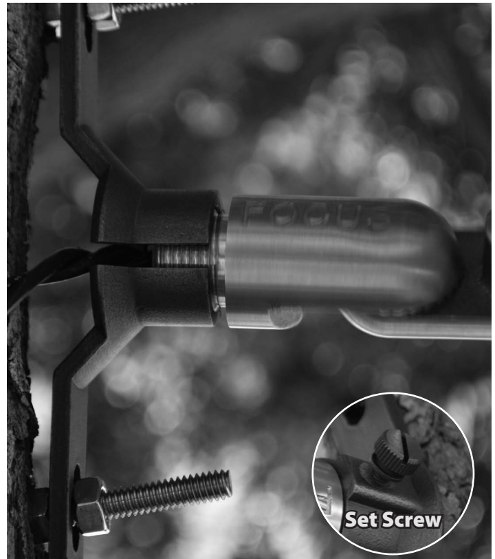
4. Run lead wire through slot & attach fixture to bracket. Use set screw to set desired fixture angle. Secure lead wire to tree and connect to main cable
